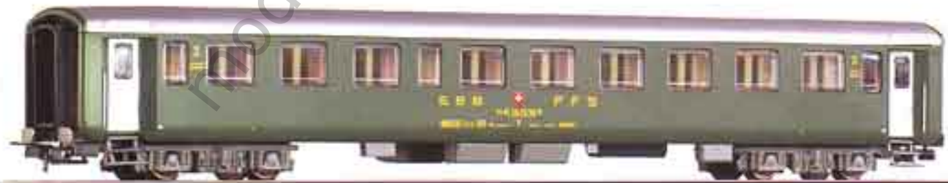
Reisezugwagen 2. Klasse, Bauart Schlieren, der SBB 2nd class passenger coach of the SBB
