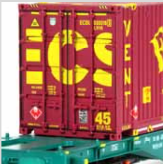
54.403 - Sgns wagon, LINEAS Belgium, with 45ft container ECS Zeebrugge : ECS container version BULK
